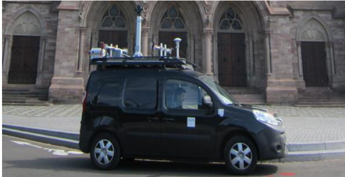
Stereopolis: multi-sensor 3D mobile mapping system for street visualisation and 3D metrology
