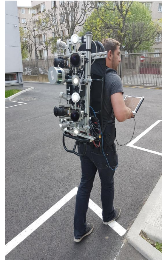
Backpack image/lidar acquisition
